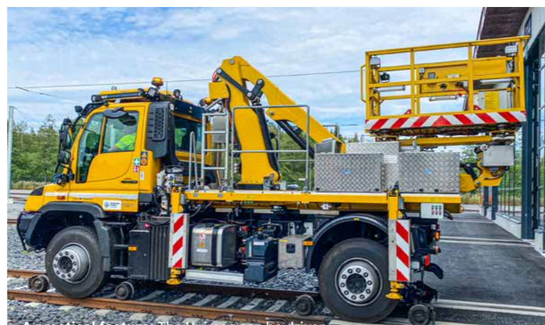
A practical feature: The Unimog can be driven remotely from the elevating work platform.
