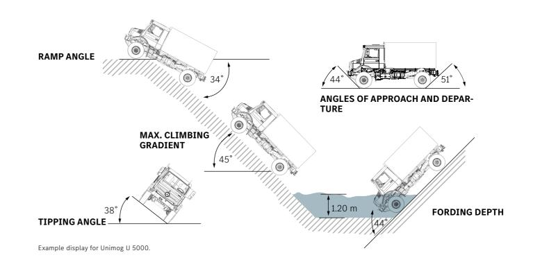
**Safety first. In any terrain.** Crossing rivers, climbing sand dunes, negotiating mud and navigating steep embankments: Mercedes-Benz trucks are famous for their innovative suspension design.
